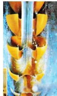
Figure 1 A large Pelton wheel with four jets, wheel and water jet that impinges the buckets.
