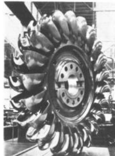
Figure 1 A large Pelton wheel with four jets, wheel and water jet that impinges the buckets.
